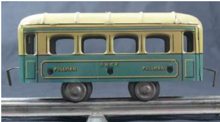
JEP 28 mm Pullman car: catalogue number 4311.V and a length of 10 cm. Made from 1938 till 1950.
