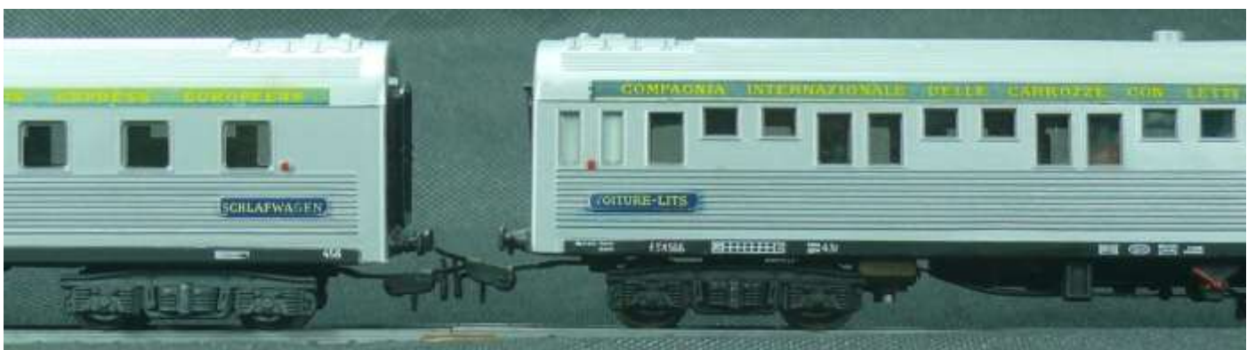
Right the coach with interior lighting, an electrical connection can be seen at the underside.
