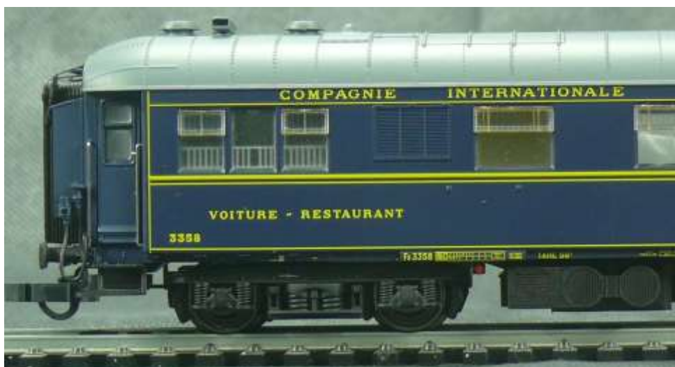
Note the air-conditioning next to the kitchen windows which was added to this WR
