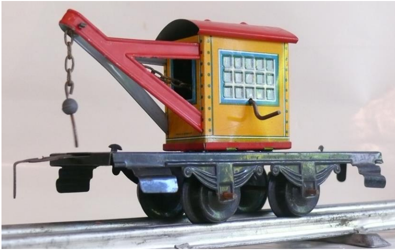
The body can be rotated and the hook lowered with the crank. The jib is fixed.
