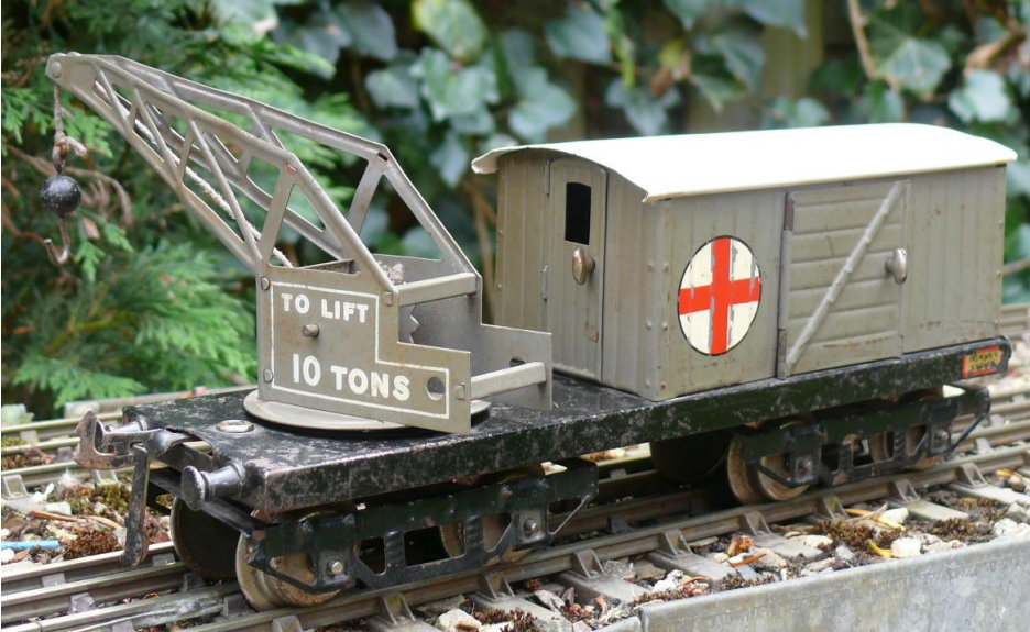
With this car, also the crane body can be rotated and a winding handle is used to raise and lower the hook.
