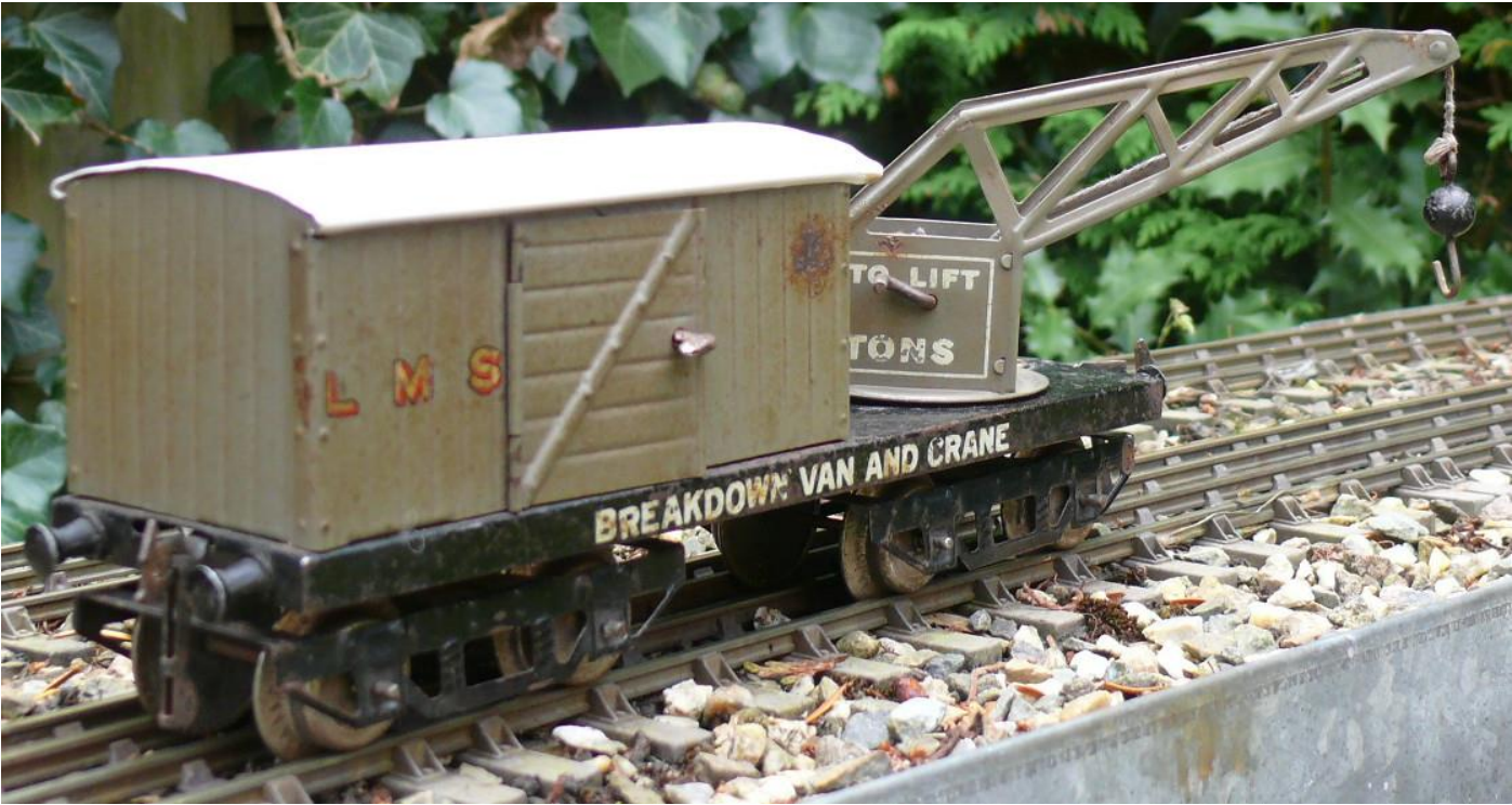
With this car, also the crane body can be rotated and a winding handle is used to raise and lower the hook.
