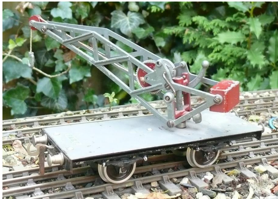
The fixed jib can be rotated and the hook lowered with a crank.
