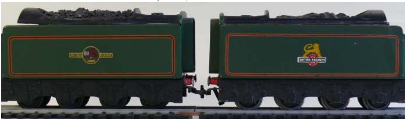
Left the 2-rail tender, right the 3-rail version. Note that the tender top of the newer 2-rail version is more deformed than the top of the older 3-rail version.
