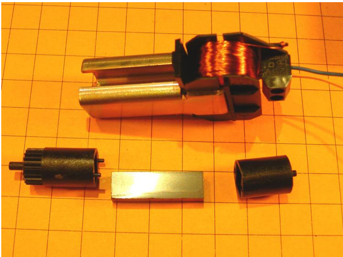
The EPL Coil with the Pole pieces attached, the bar magnet and two part case that houses the magnet, showing the gear drive for the rack.
